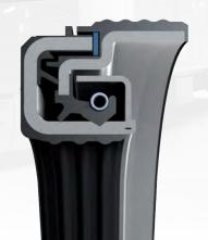
Multi-zone labyrinth construction creates superior protection and low friction. A wide inside diameter with rubber ribs ensures proper sealing. Outside-diameter seal points provide a secure fit in the hub, and thicker gauge steel protects against internal damage during installation
