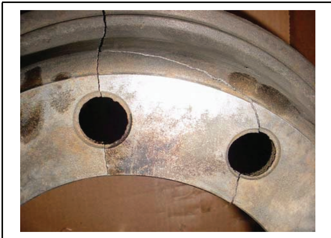
Cracked Mounting Flange FIGURE 12
