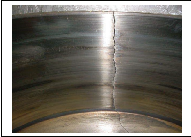
Cracked Drum Barrel FIGURE 11
