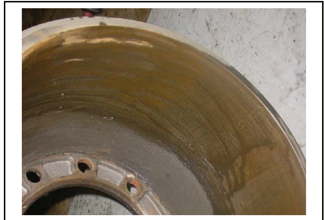
Oil-Stained Drum FIGURE 17
