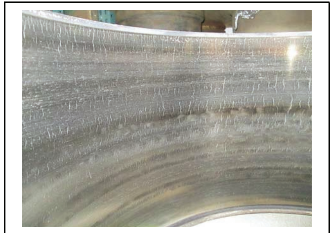
Light Heat Checks
