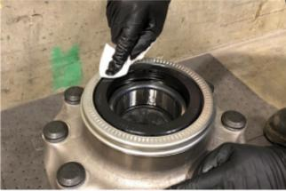
Wipe any excess lubricant off the "AIR SIDE" surface of the seal and the hub with a clean cloth.
