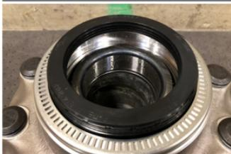
Place the seal flat on top of the seal bore chamfer, with the "AIR SIDE" visible.
