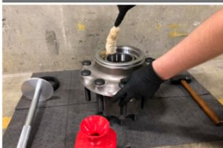
Use a clean applicator or finger to lightly lubricate the seal bore of the hub.
