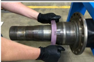
Ensure the entire seal journal is free of surface damage and debris.
