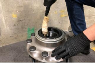
Use a clean applicator to lightly lubricate the inner diameter of the seal and the bearing cones (hub bearing lubricant or lubricant included with seal is recommended).
