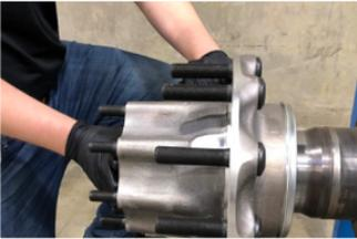
Place the outboard bearing cone in the hub and install the hub assembly onto the axle in one smooth continuous motion, while keeping the hub aligned with the axle to prevent seal misalignment.
