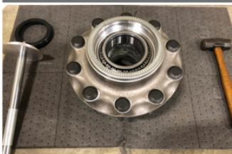
Ensure hub is sitting on a clean, flat level surface and the seal bore is free of rust, dirt, scratches, and sharp edges.
