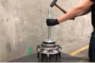
Use the appropriate ConMet seal installation plate (see table below) with a generic tool handle or a flat plate and a small mallet to hammer seal into place. Ensure the seal is uniformly bottomed out in the hub bore.
