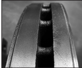
Wear Line Indicator FIGURE 120
