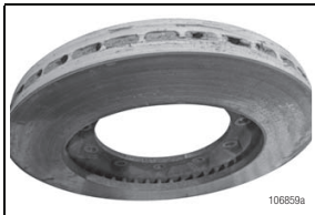
Clogged Vent Holes FIGURE 117
