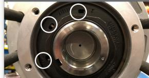
Visually examine the three holes in the face of the spindle nut. One of the holes will line up with the holes in the inner washer.
