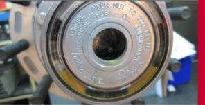
Be certain the hubcap is properly filled to the "oil level" mark on the face of the cap. Allow the initial fill amount to settle for 10 minutes. Repeat the fill procedure until the oil is at the fill line on the hubcap.
