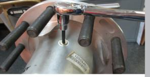
Install fill plug and torque the plug to 20 to 25 ft.-lbs.
