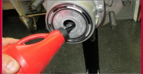
Fill the hub with oil through the hubcap or the fill hole on the barrel of the hub.
