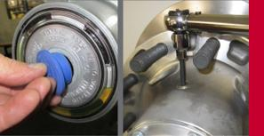
Reinstall fill plug in the hubcap or the barrel of the hub. Torque the fill plug in the barrel of the hub to 20 to 25 ft.-lbs.
