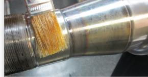
Lubricate the bearing journals on spindle or the inside diameter of the bearing cones with grade 2 grease or the lubricant that will be used in the wheel end.
