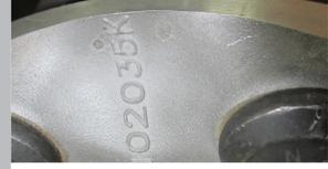
Use the casting number on the hub and the semi-fluid grease chart below to determine the proper fill volume.
