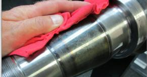
Remove any lubricant, corrosion prevention coating, foreign material or surface rust on the spindle.
