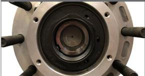
Use a smooth, firm motion and place the hub onto the spindle. When the threads on the nut engage the threads on the spindle, rotate the nut in a clockwise direction to fully engage the threads.
