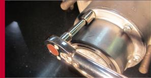
Install the hubcap and torque the bolts in a star pattern to 12 to 18 ft.-lbs.
