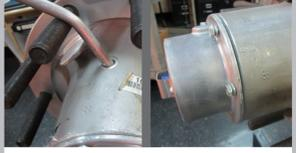
Install the hubcap, but do not tighten the bolts to allow for venting while filling. Install the semi-fluid grease lubricant through the fill hole in the barrel of the hub.
