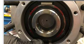
Insert the tab of the red locking snap ring through the aligned nut and washer holes. Spread the ring, push over the spindle nut and into the machined grooves. Use caution not to bend the locking ring. If the ring is bent or damaged, replace with a new one.
