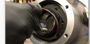
Remove the red locking snap ring from the spindle nut. Verify that the bearing spacer is in proper alignment. Align the key on the washer with the keyway on the spindle.
