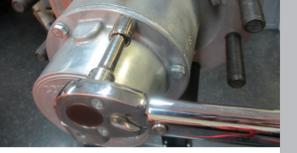
Torque the hubcap bolts in a star pattern to 12 to 18 ft.-lbs.
