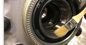
Remove all packaging, this may include outboard and inboard cardboard rings and a bungee disc. Lubricate the inside diameter of the seal with the same lubricant that will be used in the wheel end.
