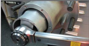
Torque the spindle nut to 500 ft.-lbs. while rotating the hub.
