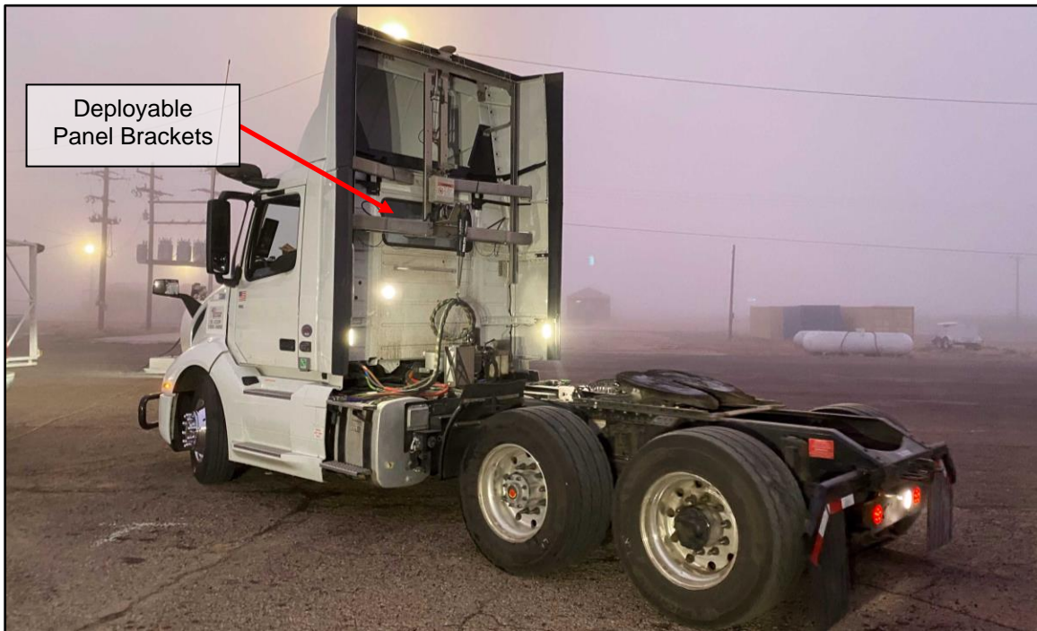
Figure 5: Baseline Configuration with TruckWing Panels Removed
