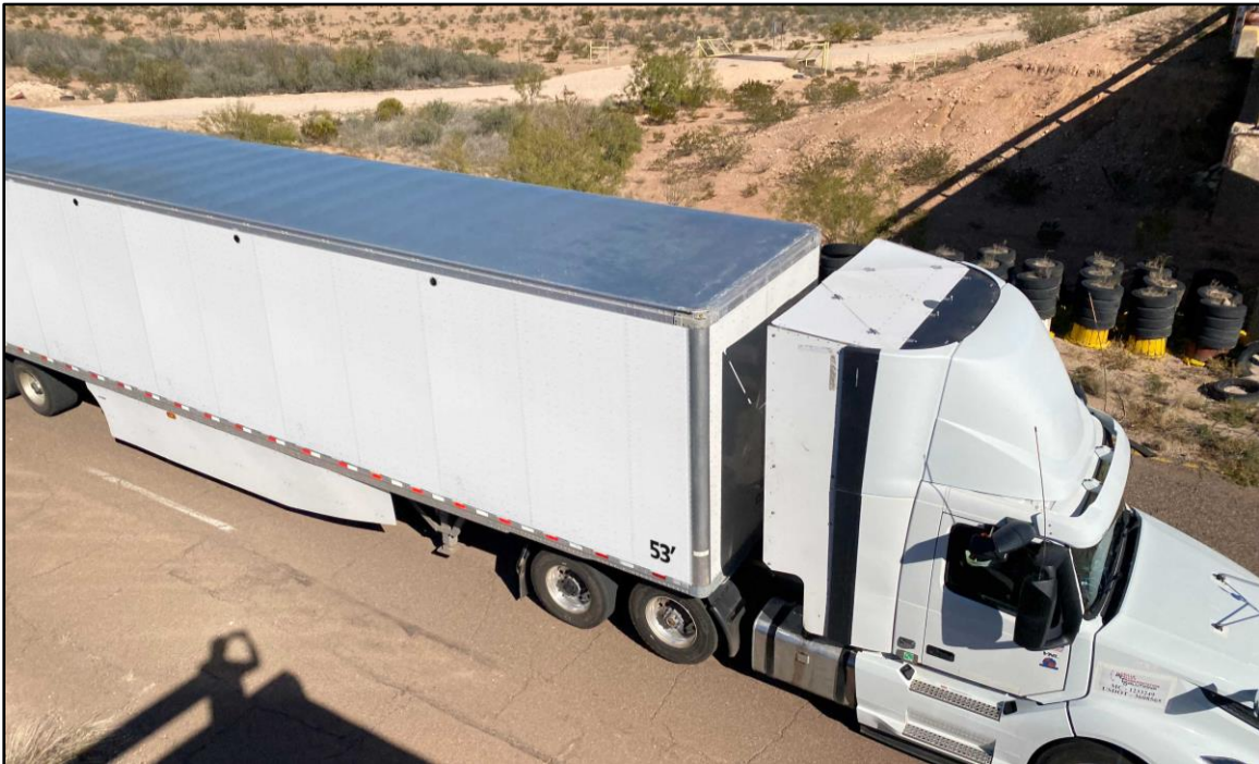
Figure 4: ConMet TruckWings™ Deployed at Speed
