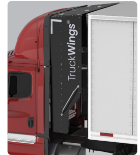
Speed > 52 mph panels deploy
