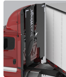
Speed < 50 mph panels retract
