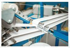
Greif® GCore tube winding adhesives are formulated to meet your needs and designed to run on your equipment. Greif offers clay-filled and non-filled (resin) types, and capabilities include bonding difficult paper, grease-proof and plastic plies and providing heat and/or water resistance.
