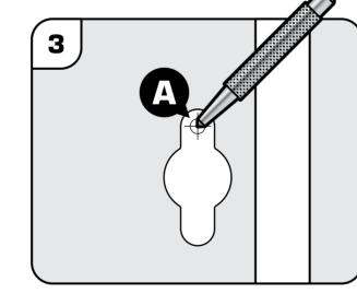
Use a centre-punch to punch the centres of the mounting points (marked 'A'). Note, all four Mounting Points must be used.
