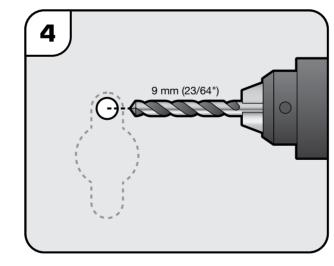
Remove the Template then drill clearance/pilot holes using a 9 mm (23/64") drill bit (or drill bit size for your chosen fasteners). De-burr the holes and touch up any bare metal surfaces that have been exposed with a rust inhibitor (e.g. primer).
