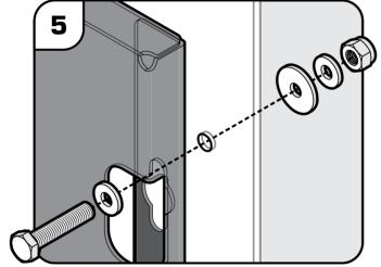
Fasten the ICMS-010 in place using your chosen fasteners. Get someone to help you lift and locate the unit safely if needed.
