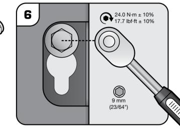
Torque to 24.0 N·m/17.7 lbf·ft if using the recommended fasteners, or torque appropriately for your chosen fastener grade.
