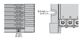
REDARC recommends using six M6 (1/4") bolts/screws with washers. If using countersunk fasteners, apply countersunk washers to avoid damaging the Mounting Points.
