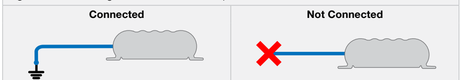
Figure 10: Connecting the BLUE wire to solar panel
