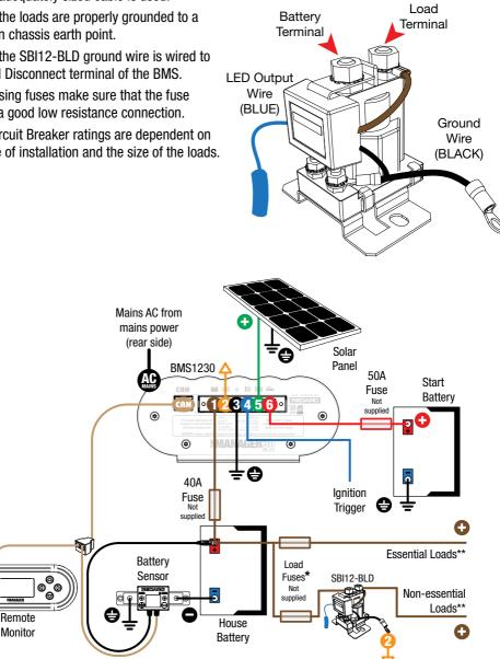
\* The size of this fuse relates to the total current draw of all the loads connected to the House Battery, and should be rated slightly higher than this.
