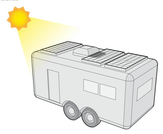
Be aware of shading that can occur as a result of roof mounted accessories on your caravan or motor home. Shading sections of your solar panels will significantly reduce your solar panels performance.
