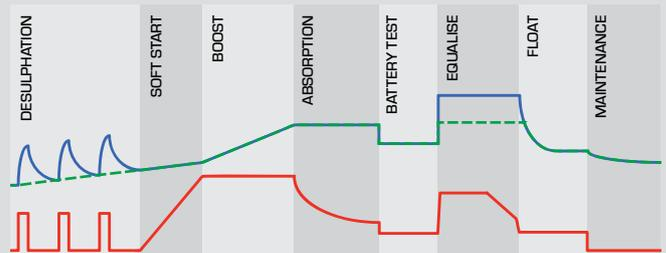
Sophisticated fault detection sensors monitor the battery conditions during all stages of charging, keeping you and your caravan/camper safe.
