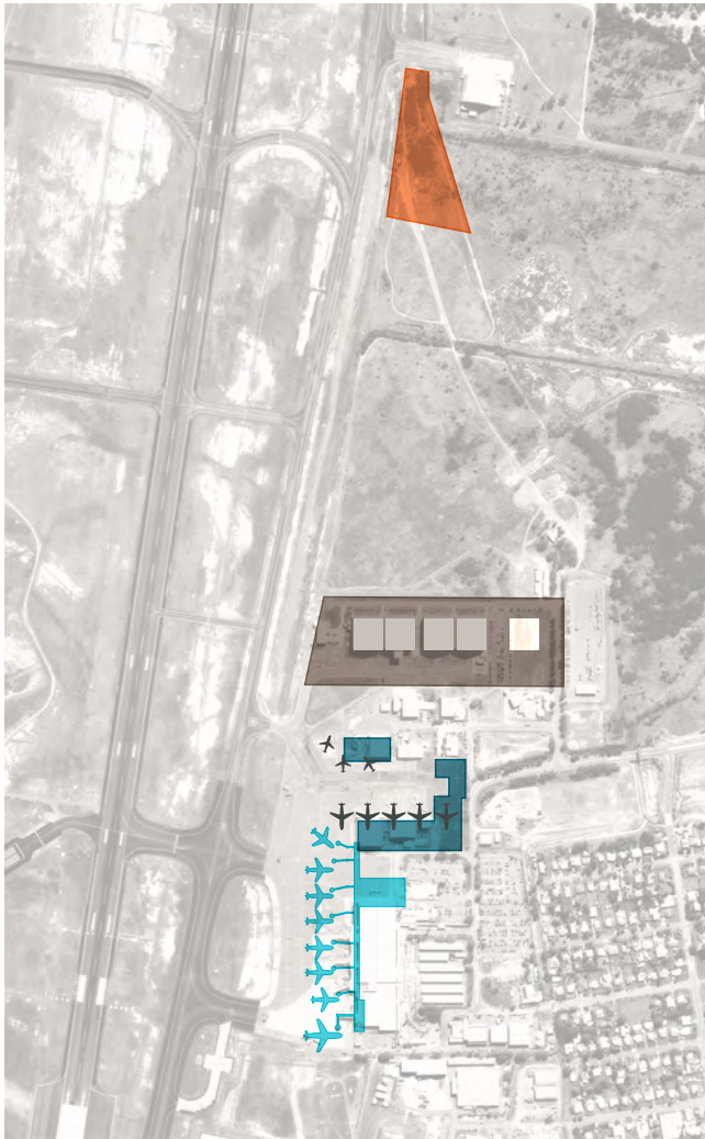
Figure 3.2.1.4 — Initial (8-yr) Airfield Development
